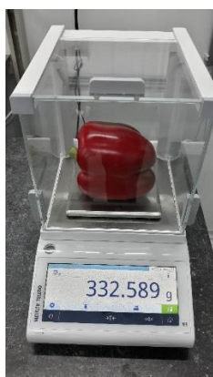
Figure 6 Weighing individual peppers on three digit scale with chamber
