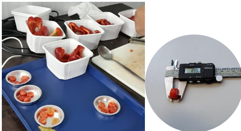
Figure 10 Preparing discs (left), measuring thickness (right).
