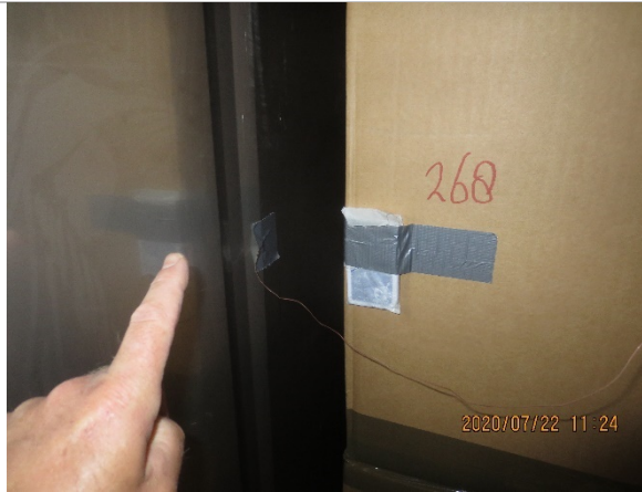
Figure 28 Wall surface temperature measurement near sensor 268.
