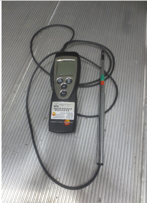
Figure 19 Handheld hot wire anemometer used to assess supply air flow rate.
