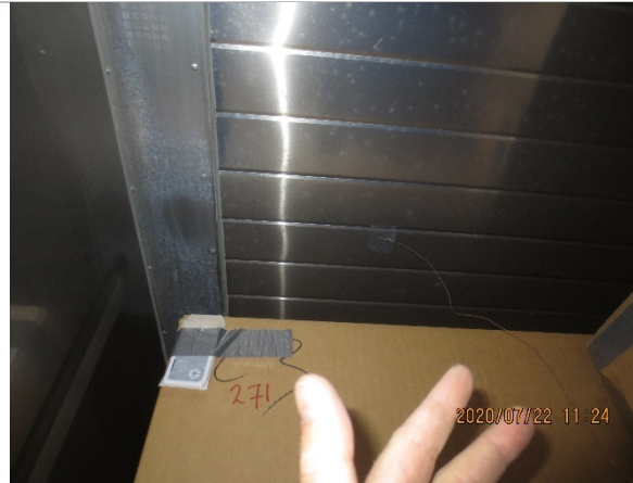
Figure 29 Cceiling surface temperature measurement near sensor 271.
