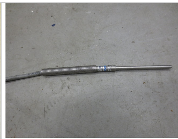
Figure 17 ATP sensor (= 4-wire PT100 temperature sensors of IEC751 class A, manufacturer: Tempcontrol).
