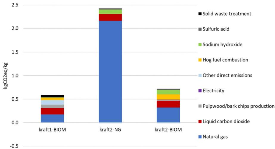
**Fig. 2.** Cradle-to-gate climate change impact (excl. biogenic carbon removal) of 1 kg of kraft lignin. Biogenic carbon content expressed in terms of carbon dioxide equivalent: 2.4 kg CO<sub>2</sub>eq/kg.
