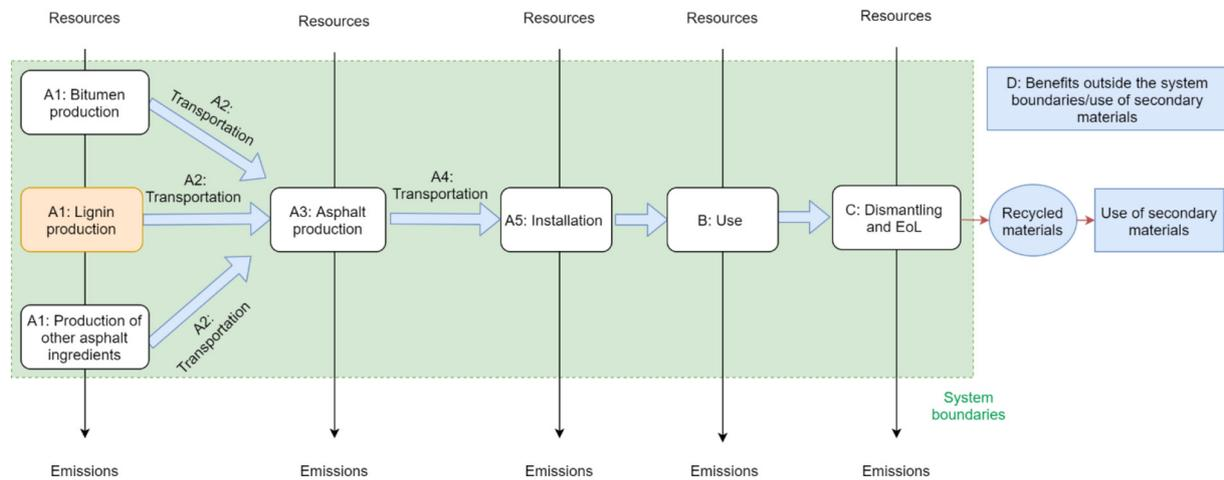
**Fig. 1.** Flow chart of lignin-based asphalt with cradle-to-grave life cycle stages based on (Schwarz et al., 2020). The unit process named “A1:Lignin production” starts from the cradle to the gate of the pulp mill where lignin is delivered.
