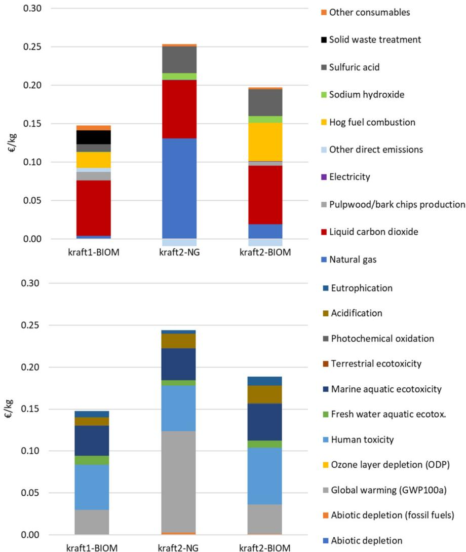
**Fig. 3.** Cradle-to-gate MKI score of 1 kg of kraft lignin. Breakdown per process contribution (top bars) and impact category (bottom bars). In this figure, the MKI score is without biogenic carbon removal, which accounts for 0.12 €/kg.
