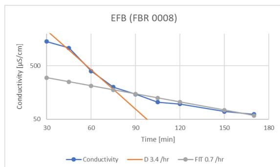
**Figure 2:** Conductivity profile for single column EFB extraction
