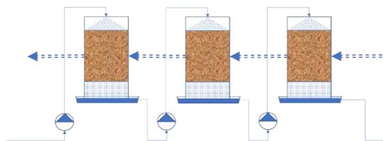
**Figure 1:** CC SMB Extraction Setup
