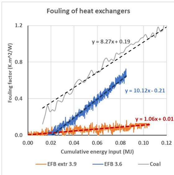
Figure 4: Combustion tests (heat exchanger fouling)
