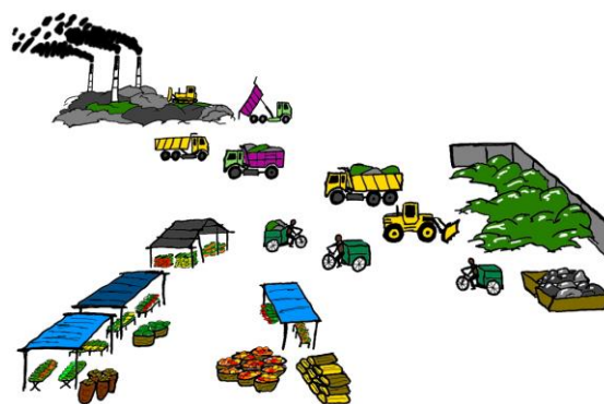
Figure 1: Current waste disposal: collection and disposal of waste from fresh markets. Waste is collected and transferred to the secondary transfer station using vans. The waste is transported from the secondary transfer station to the landfill using trucks.
