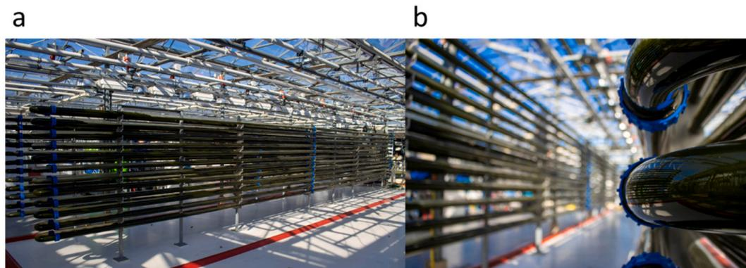
**Fig. 1.** LGem tubular photobioreactor (PBR) used for the pilot-scale production of *N. oceanica*. Se-enriched biomass: (a) 1500 L tubular PBR system. (b) close up of the glass tubes of the LGem system. Pictures were taken in AlgaePARC, Wageningen University and Research, The Netherlands.
