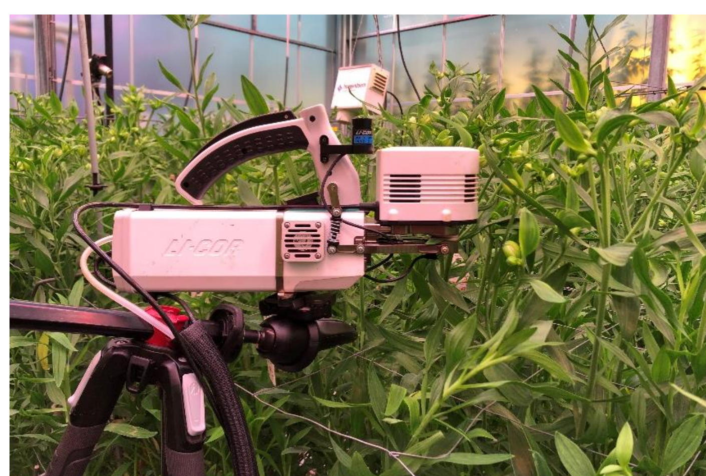
Figure 2. Li-6800 during photosynthesis measurements.
