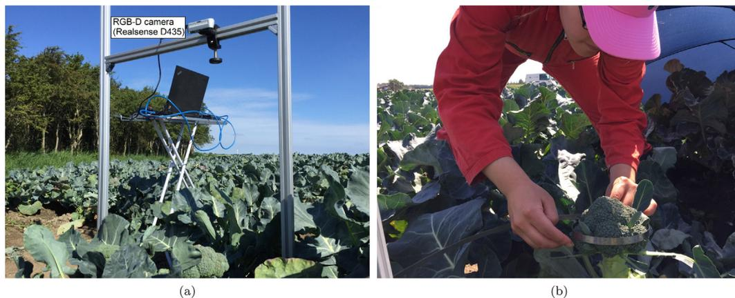
**Fig. 3** – (a) The Intel Realsense D435 camera was mounted on a metal frame to acquire top-view RGB-D images of broccoli heads in a field in Sexbierum (The Netherlands). (b) After the image acquisition, the diameter of the broccoli head was measured with a circular ruler.
