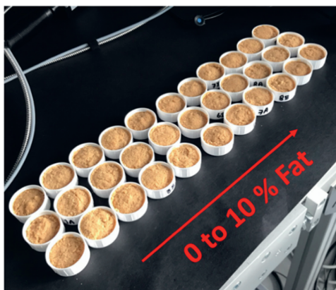
Figure. 9.1. Prepared samples with known fat content as used for NIRS measurements.
