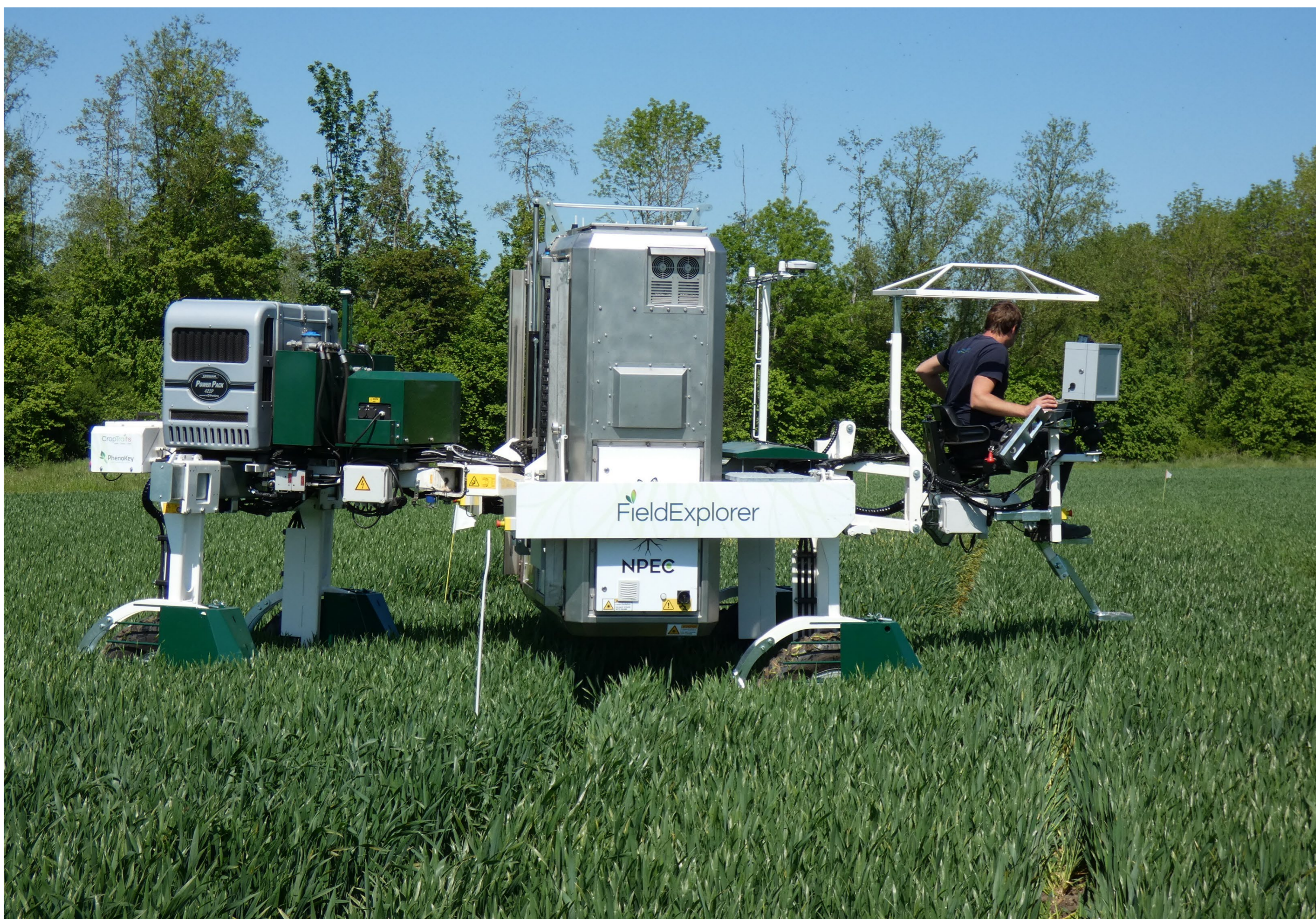
Figure 1. TraitSeeker from the Netherlands Plant Eco-phenotyping Centre (NPEC) is taking hyperspectral images of the experimental fields at SPNA on 31 st May 2021. TraitSeeker carries two hyperspectral cameras, one RGB camera and one laser sensor. It is operated by Unifarm from Wageningen University & Research.
