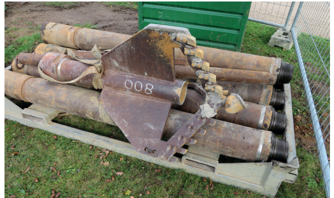
Fig. 2: Drill head for the well shafts (approx. 80 cm diameter).
