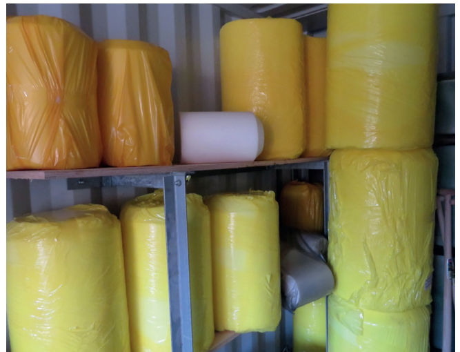
Fig. 6: Various sizes of foam pig waiting, ready to clean out the pipes.
