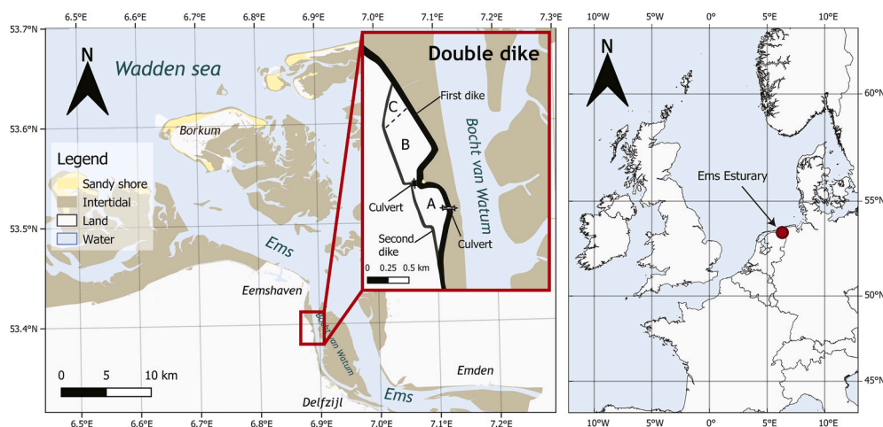
Fig. 2. The location of the Double Dike between Eemshaven and Delfzijl within the Ems estuary. Sections A, B, C are the different zones planned for different functions, each connected by culverts to the sea. Base map adapted from OpenStreetMaps
