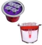
Vittorio Saggiomo at the laboratory of BioNanoTechnology came up with the device together with Professor Aldrik Velders. The CoronaEspresso uses the LAMP (Loopmediated AMPlification) technique to detect genetic virus material. Like the PCR test, this technique is much more sensitive than conventional antigen self-tests, says Velders. 'Usually, only severely infected people test positive with an antigen test.'
