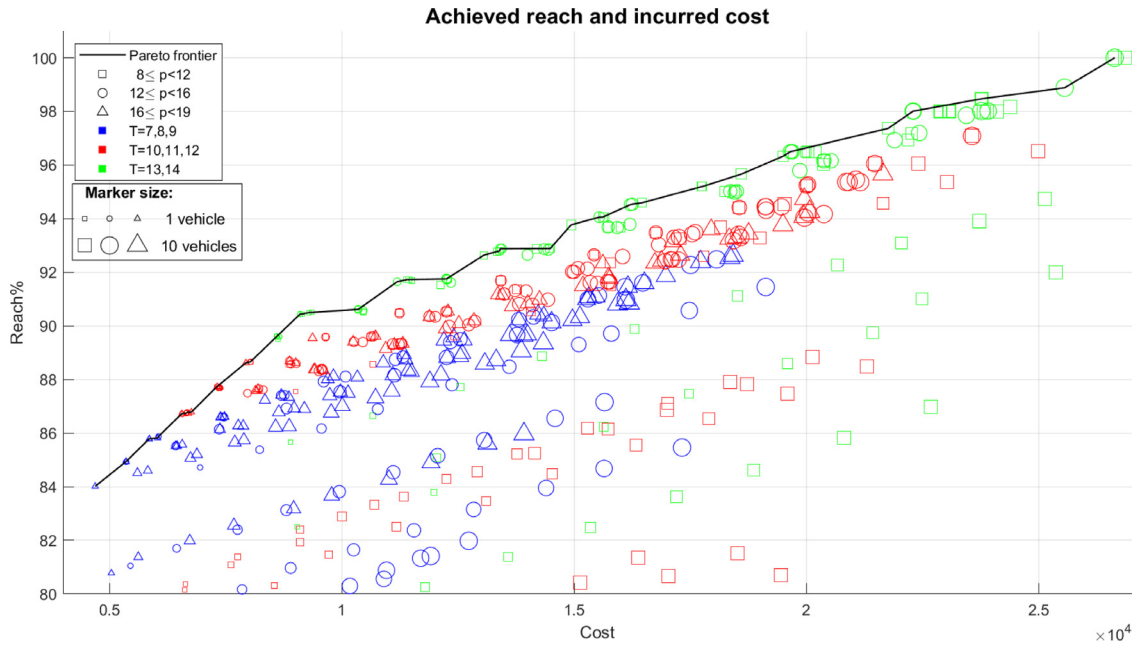
Fig. 6. Cost-Reach trade-off for different nominal capacities: (T, p) . Marker sizes are proportional to the number of vehicles..
