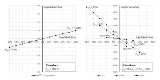
**Figure 9.** Sensitivity analysis of four parameters. Left:  $P_{ATES}$ . Right:  $\eta_2$ ,  $\eta_{rec}$  and  $\eta_{car}$ .
