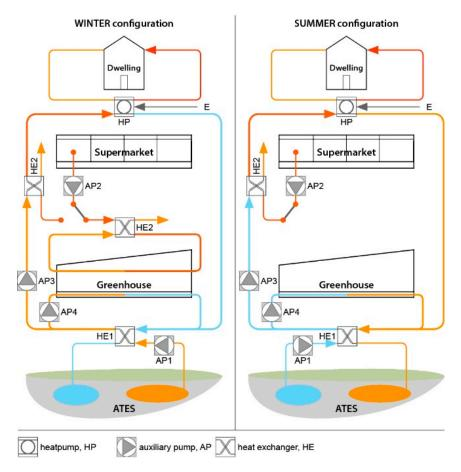
**Figure 6.** Position of the Auxiliary pumps (AP), Heat exhangers (HE) and Heat Pumps (HP) within the local energy system for both system configurations.
