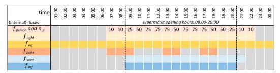
Figure A1. Hourly timetable of time based thermal fluxes for the super-market building.
