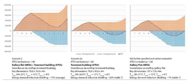
**Figure 7.** (Dis)charging of the ATES. Both the tenement building as the gallery building can be heated by means of a rooftop solar collector, provided that the system is configured under specific climate settings. Scenario 2 & 2a correspond with the scenarios described in Section 3.4.
