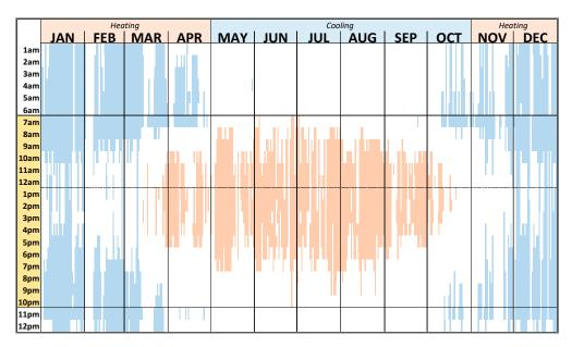
**Figure 4.** Indoor Greenhouse temperature ( $^{\circ}$ C). Initial set point temperatures:  $T_{max} = 28 \, ^{\circ}$ C,  $T_{min-D} = 9 \, ^{\circ}$ C,  $T_{min-P} = 12 \, ^{\circ}$ C. Blue indicates that  $T_{min}$  has been reached or supassed, red indicates that  $T_{max}$  has been reached or surpassed and white indicates that the GH indoor temperature is within desirable range. The yellow hatched hours indicate the photoperiod (PP) timeslot.
