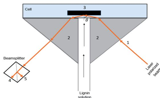
Fig. 1 Schematic illustration of the SPAR experimental set-up.
