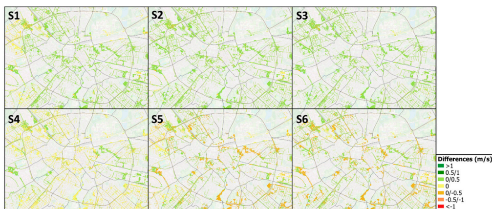
Figure 11. Differences in flood velocity under NBS scenarios (S1 to S6) relative to baseline for 100-year return period.
