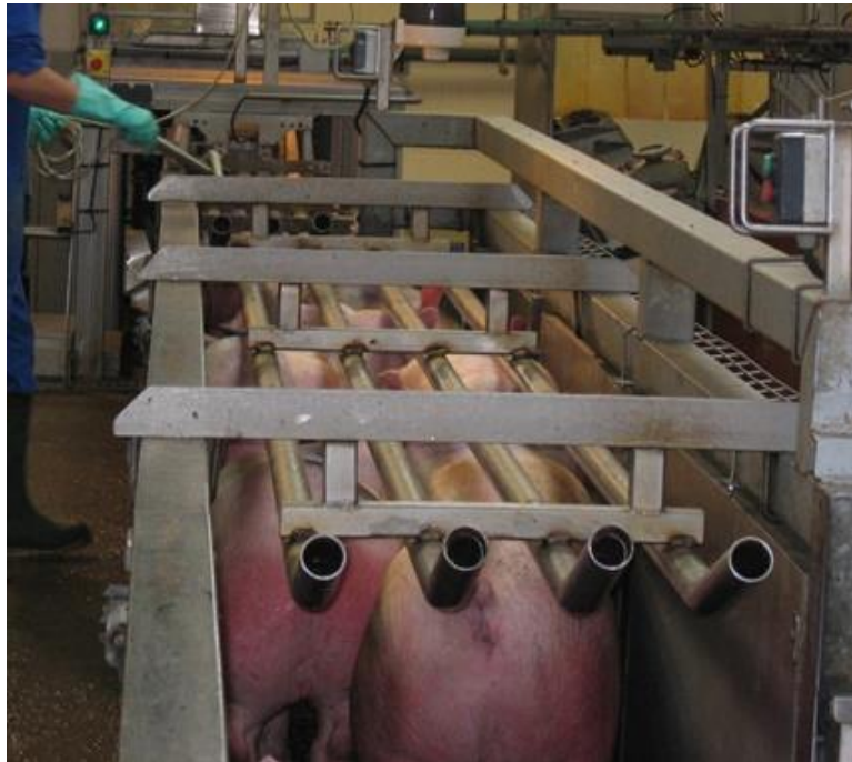
Figure 3.1.2. Moving pigs in lines in the raceway to the electrical stunner (© V. Michel, 2019)
