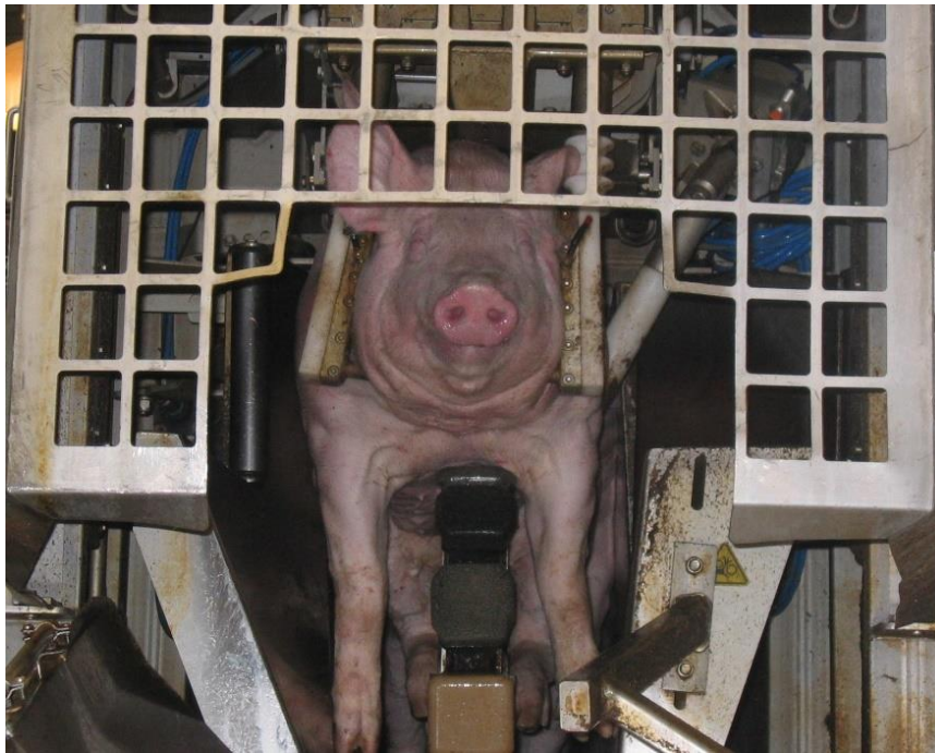
Figure 3.2.4. Head-to-body stunning on a breast band conveyor restrainer. The electrodes are placed while the belt continues to move forwards (© A. Velarde, IRTA)
