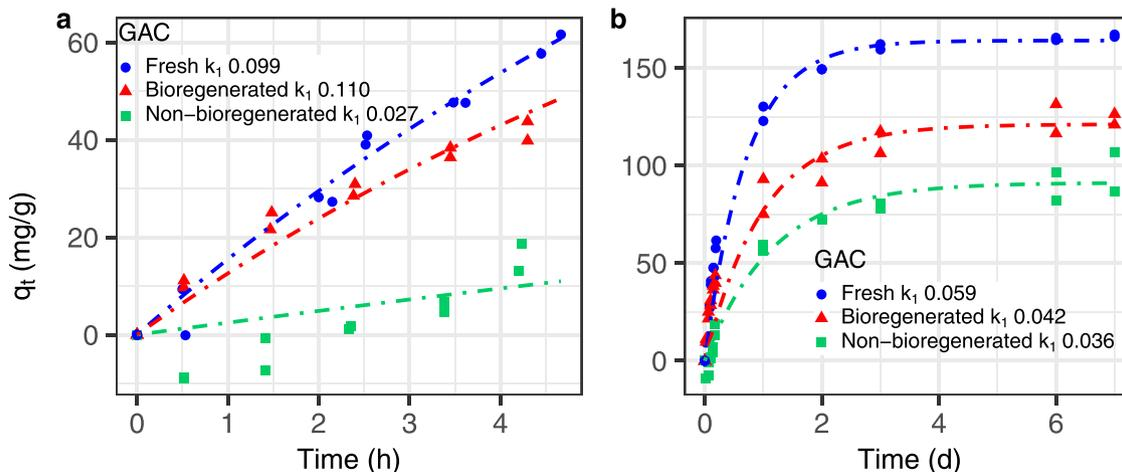
Fig. 8. Melamine adsorption by fresh and bioregenerated GAC abiotic control and respective first-order adsorption constant ( $k_1$  in 1/h) in the period. a: First 4.5 h of adsorption. b: 7 days of adsorption. Data points represent experimental data. Lines represented fitted pseudo-first order kinetics equation (Eq. (7)).
