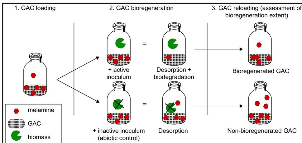
Fig. 2. Schematic representation of steps in GAC bioregeneration experiment.
