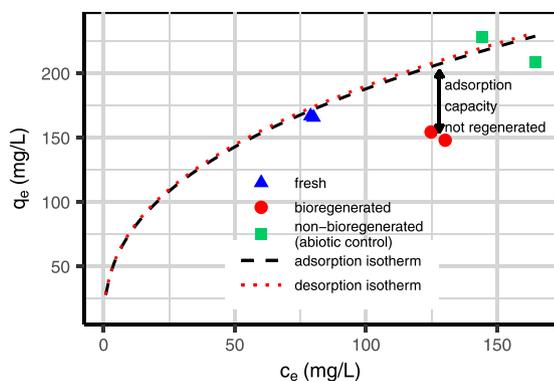
Fig. 7. Melamine load on fresh GAC, bioregenerated GAC and abiotic control compared to the expected load based on the adsorption and desorption isotherms. Duplicates are plotted individually.
