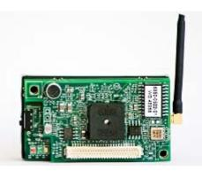
Figure 3: Wireless Multi-Sensor Nodes are Starting to Integrate GPS Technology which Enables Geolocation of the Nodes and their Data.
