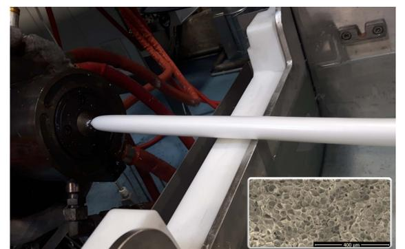
**Figure 3.** Stable foam production at Sulzer. SEM example of a foam structure.
