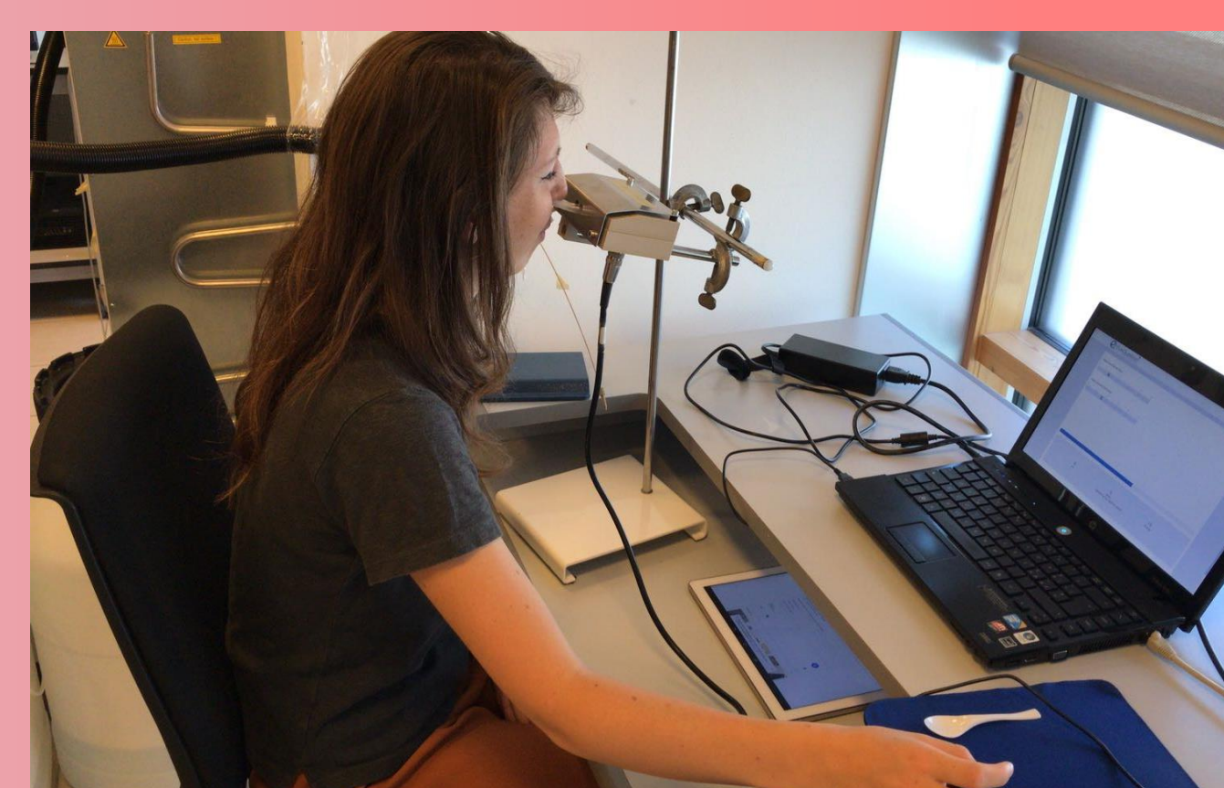
Fig. 1: Example of experimental set up. Participants in-nose breath was collected during chewing gum consumption and sensory evaluation.
