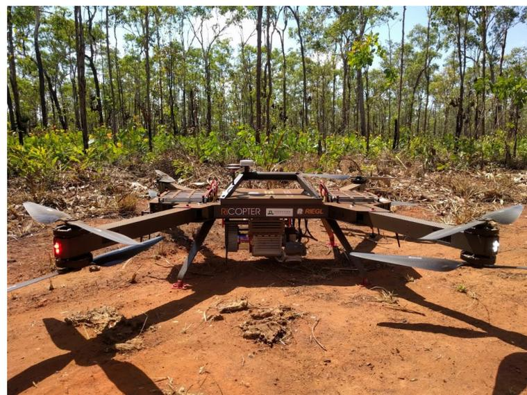
**Figure 2.** RIEGL RiCOPTER with VUX-1UAV.
