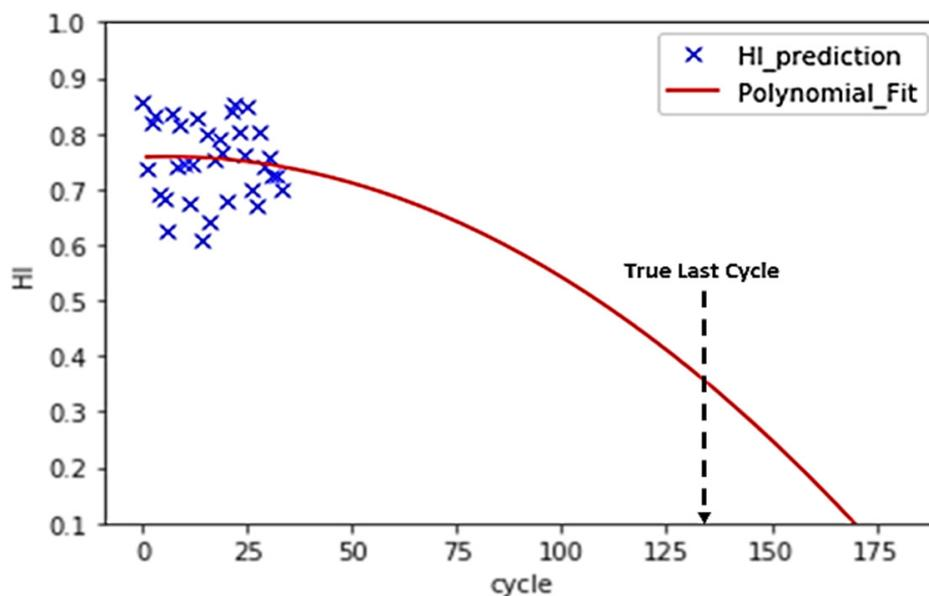
**Figure 13.** FD001\_Test turbo unit 85 (34 cycles) test data validation.
