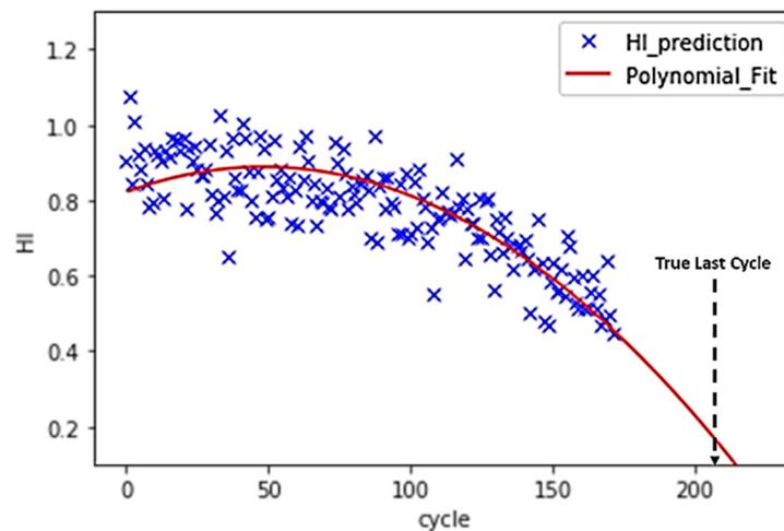
Figure 14. FD001\_Test turbo unit 84 (172 cycles) test data validation.
