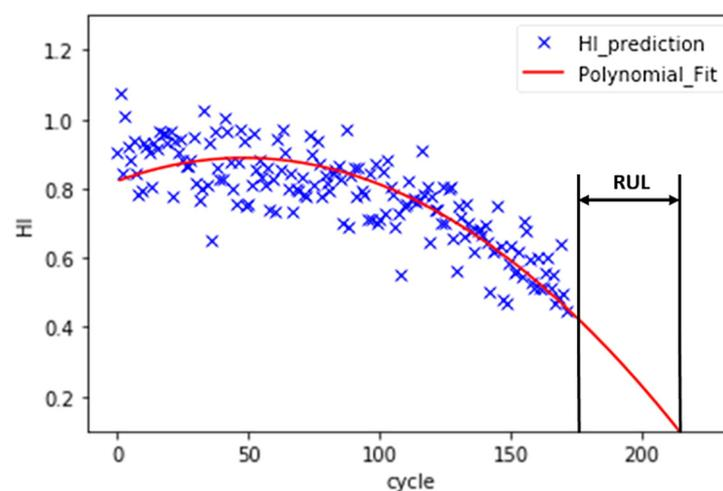
Figure 7. The HI prediction and RUL estimation for FD001\_test turbo engine unit 84.
