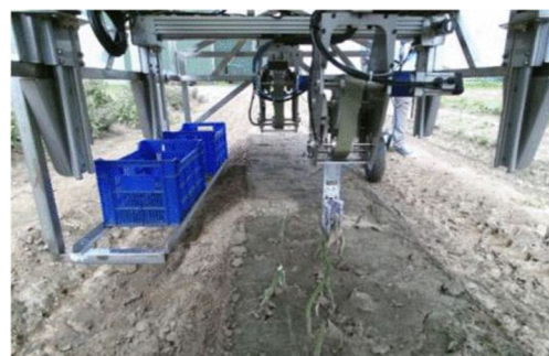
Fig. 5 A close-up of the end-effector that harvests the green asparagus
