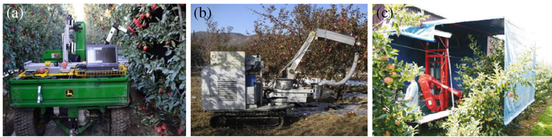
Fig. 4 Examples of apple-harvesting robots. a WSU apple picking robot (From: Silwal et al. [19], with permission from John Wiley and Sons), b JSU apple harvesting robot (From: Zhao et al. [20], with permission from
