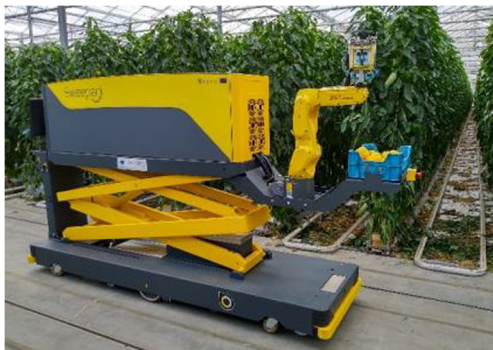
Fig. 2 Prototype of the sweet-pepper-harvesting robot SWEEPER
