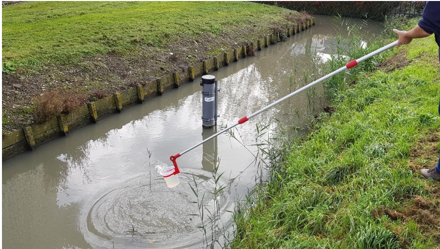
Figure 17. Continuous water quality monitoring (EC) and water sampling for lab-analysis.
