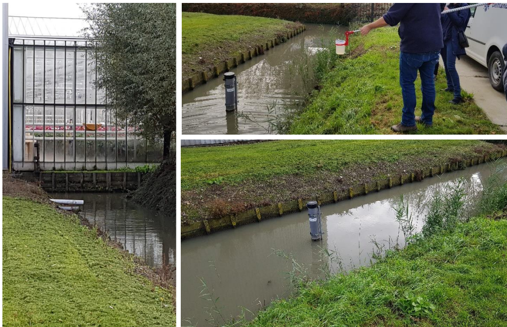
Figure 8. Traditional pipes leaching to the ditch (left). Sampling by Delfland Water Authority (right top). Fixed measuring point in a ditch to measure NPK (right bottom).
