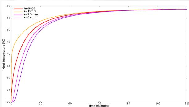
**Figure 1.** CFD simulation of the temperature field within the meat during cooking. Scan the QR code for a link to the video.
