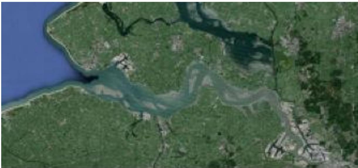
*Figure 1. The Western Scheldt with many tidal flats is the main shipping route to the port of Antwerp (right lower corner). The depth of the main shipping channel is maintained by dredging. Part of this dredged material is then replaced to the tidal flats in order to enhance the natural value of the system (source: Google Maps).*
