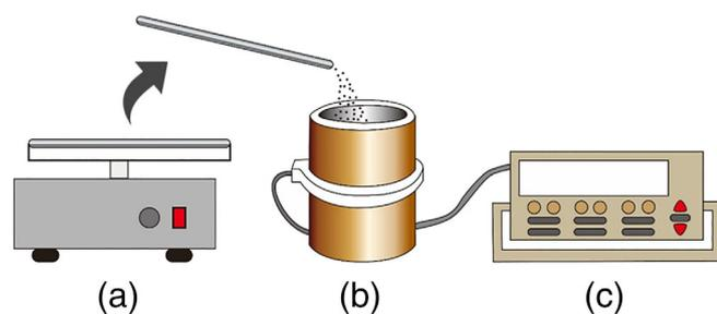
**FIGURE 3** The charging measurement system: a vibrator with charging tubes fixed on it (a), a Faraday cup (b) connected with an electrometer (c)
