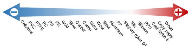
**FIGURE 1** Triboelectric series of some common materials (Liu, Zheng, Yang, & Tao, 2018; Zou et al., 2019)
