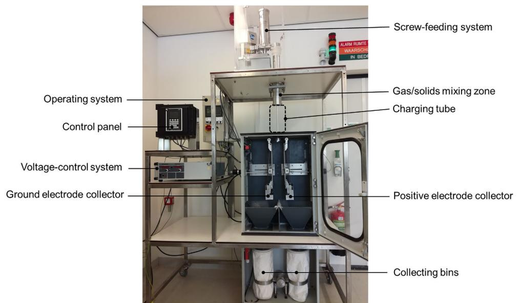
**FIGURE 2** The custom-built electrostatic separator. Main parts of the separator are indicated in the picture
