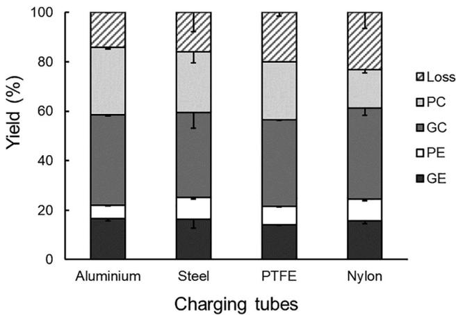
**FIGURE 7** Electrostatic separation of model mixture with different charging tubes (8 mm of diameter): yield (g/100 g flour) of four fractions collected from ground electrode (GE), positive electrode (PE), ground collector (GC), and positive collector (PC). Weight of loss was calculated by difference. The error bars represent SD, only minus direction is shown
