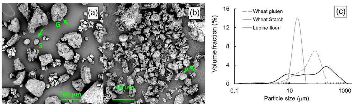
**FIGURE 5** Scanning electron microscopy picture of gluten-starch mixture (a) and lupine flour (b). “S,” “G,” and “P” indicated by arrows represent starch granular, gluten particle and protein body, respectively. The particle size distribution curves of pure gluten, starch, and lupine flour are plotted together (c)
