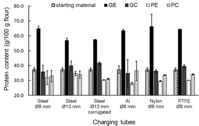
**FIGURE 8** Electrostatic separation of lupine flour with different charging tubes: protein content (g/100 g flour) of starting material and four fractions collected from ground electrode (GE), positive electrode (PE), ground collector (GC), and positive collector (PC). The error bars represent SD
