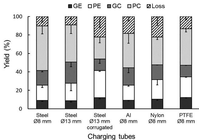
**FIGURE 9** Electrostatic separation of lupine flour with different charging tubes: yield (g/100 g flour) of four fractions collected from ground electrode (GE), positive electrode (PE), ground collector (GC), and positive collector (PC). Weight of loss was calculated by difference. The error bars represent SD, only minus direction is shown
