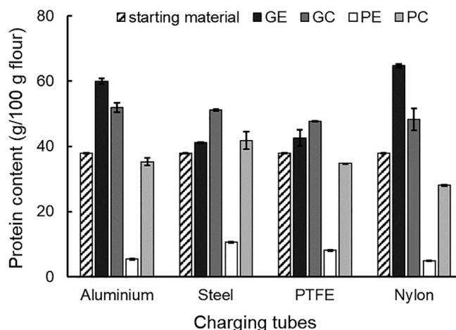
**FIGURE 6** Electrostatic separation of gluten and starch mixture (1:1): protein content (g/100 g flour) of starting material and four fractions collected from ground electrode (GE), positive electrode (PE), ground collector (GC), and positive collector (PC). The error bars represent SD
