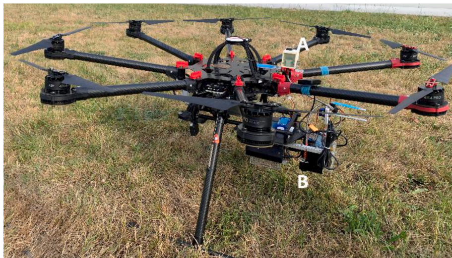
Fig. 5. DJI S1000 octocopter UAV platform with the FluorSpec mounted. “A” refers to the FluorSpec irradiance sensor and “B” refers to the radiance sensor.
