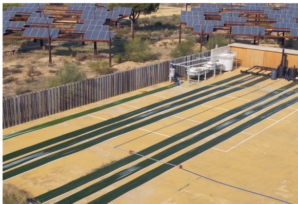
Fig. 6-2 The two out-door photobioreactors on the 27.11.2011. In front, the 6 lanes belonging to the 6 \text{ m}^3 reactor; in the back the single lane of the 600 L reactor, used for producing starter culture for the 6 \text{ m}^3 reactor. The tube crossing the 3 front lanes is the harvest line
