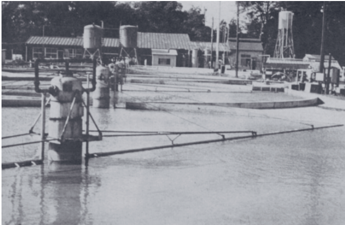
Fig. 1-1 Centre-pivot algae ponds at the Japanese Microalgae Research Institute, at Kunitachi, Japan. The pivot drives a boom that mixes the culture. (Krauss 1962)
