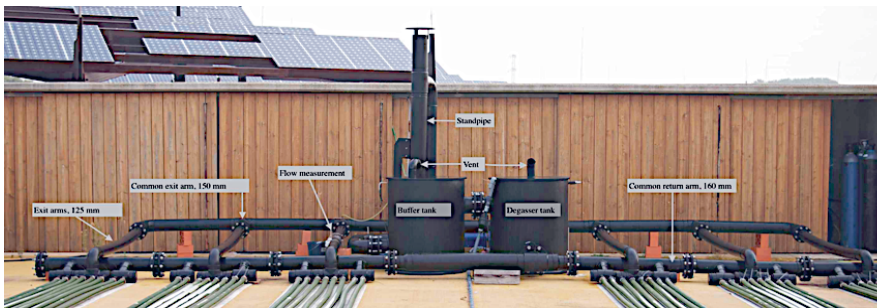
Fig. 6-3 The photobioreactor flow distribution system
