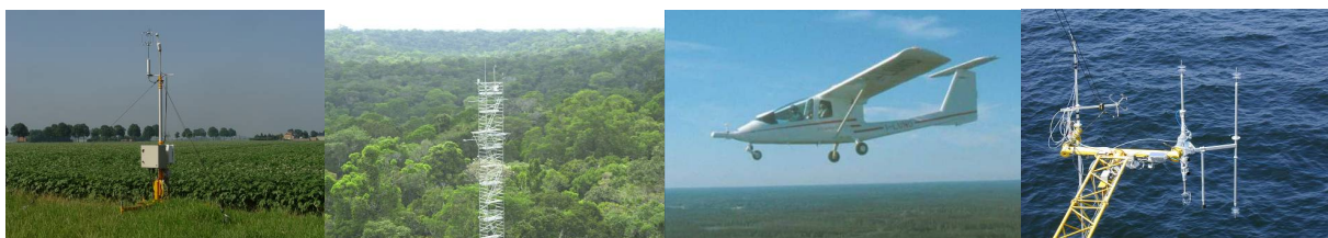
Figure 5. Examples of platforms for EC measurements. From left to right: small, quasi-mobile mast in agricultural area; fixed mast in tropical forest; research airplane; boom at the former Sample site Noordwijk. Photos: Wageningen Environmental Research.
