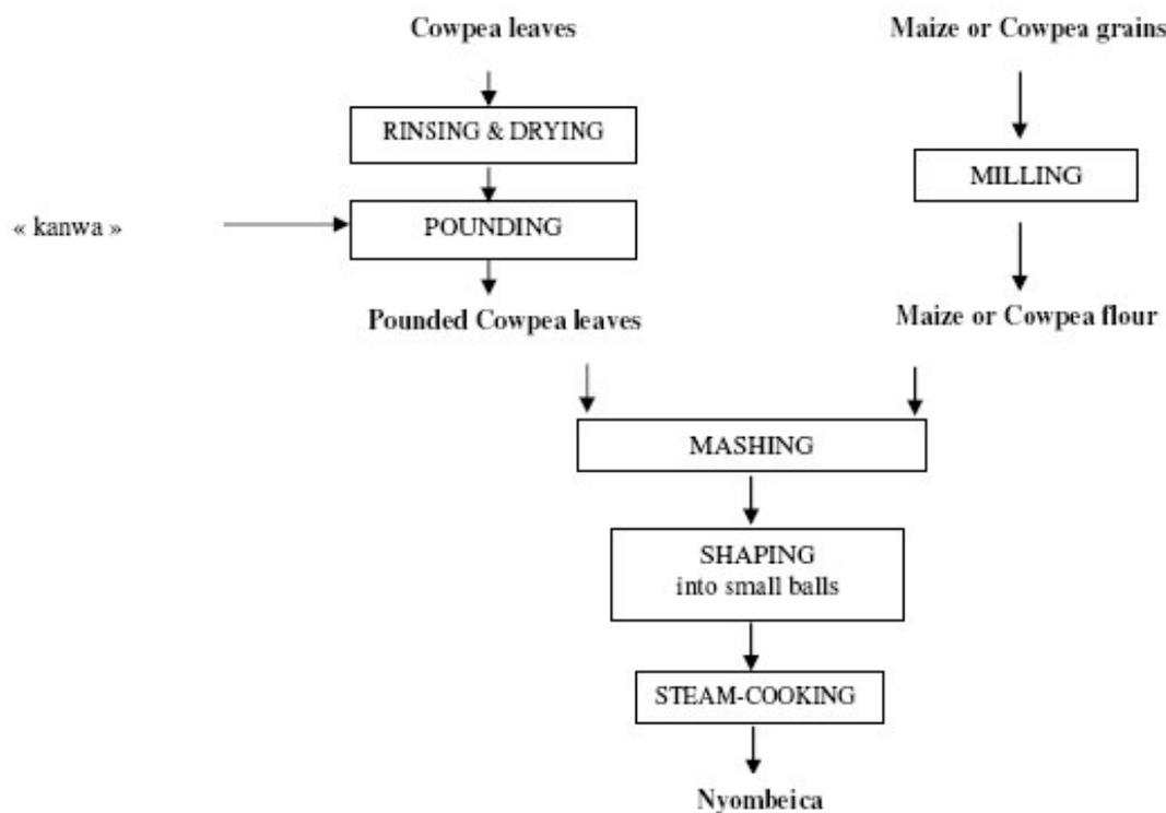
**Figure 5.** Flow diagram for Nyombeica processing.
