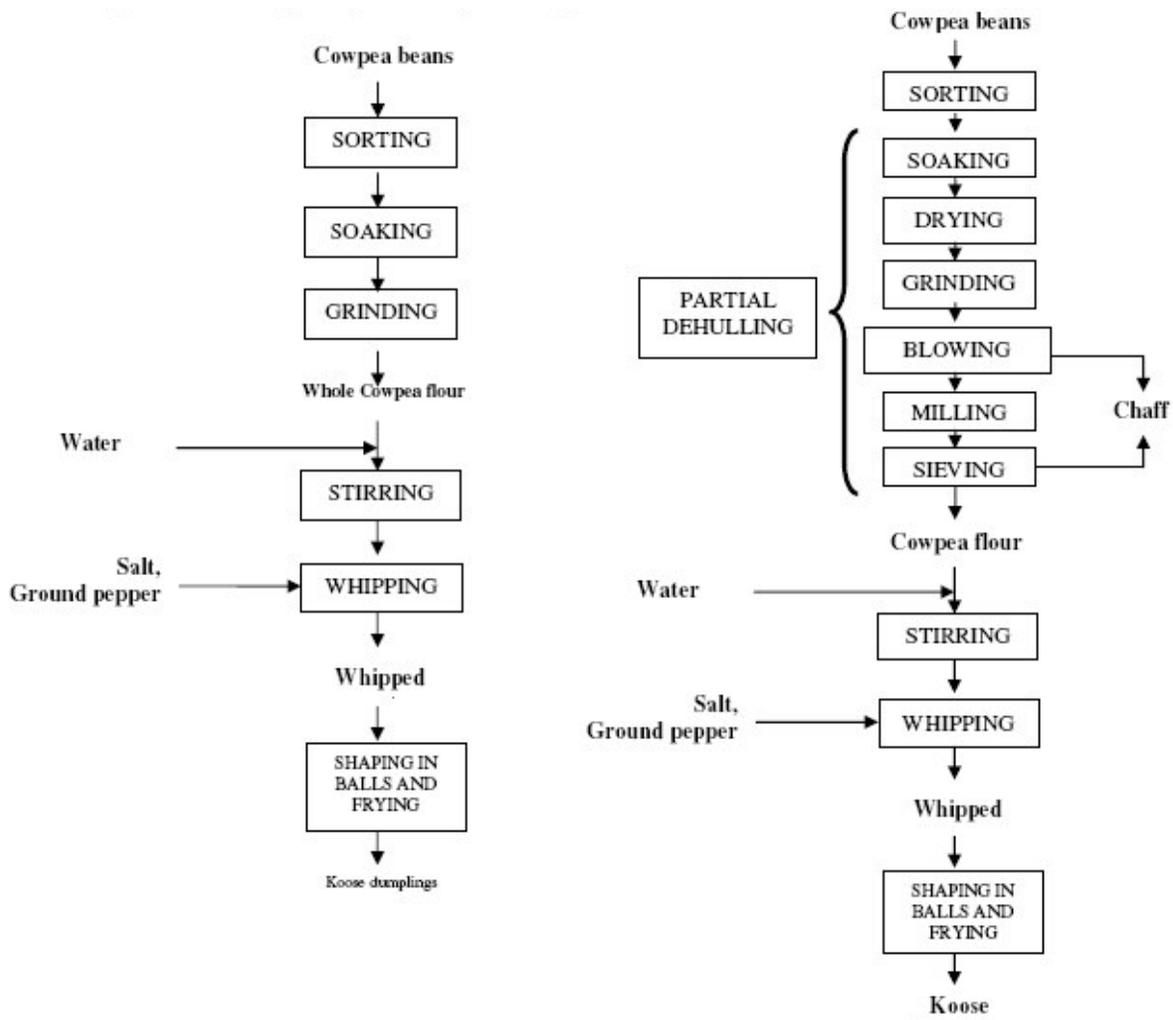
Figure 4. Flow diagrams for koose processing.
