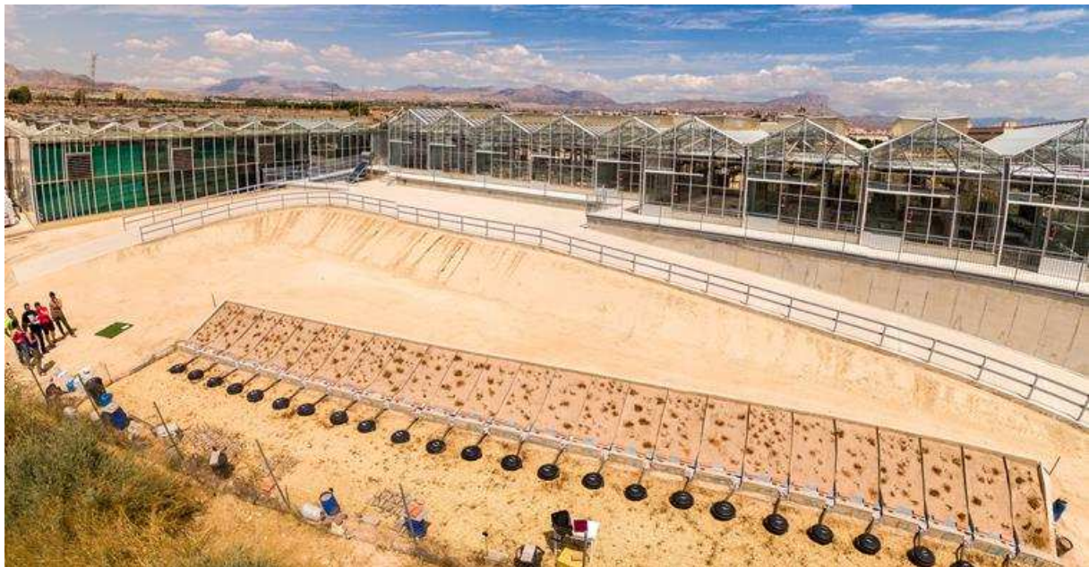
Figure 2. Aerial view of the experimental station ES24 located at the University of Alicante (Spain), showing the 24 (2x1 m) closed plots of ES24, including runoff and sediment collectors, and the greenhouse facilities in the area. Photo by D. Fuentes.
