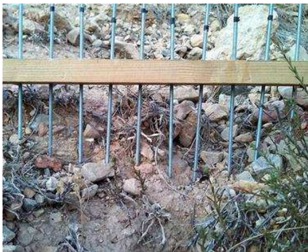
Figure 6. Two-dimensional microprofilemeter used for the monitoring of the shape of the rills developed on the experimental plots.
