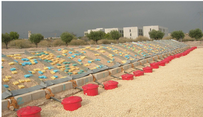
Figure 2. General view of the cover/pattern experiment using inert materials (sponges) to mimic vegetation patches (left) and detail of one large (400 cm 2 ) patch (right).
