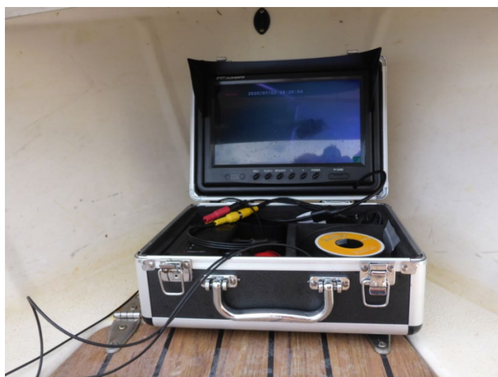
Figure 4 Eyoyo™ fish finder set up (TFT monitor) for live feed allows to control orientation and position of the baited system, as well as enables a direct observation.
