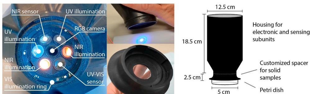
Fig. 1. Pictures and schematic diagram of the 'PhasmaFood' device: left the sensing node, middle top the handling of the prototype, middle bottom the customized spacer for measurements of solid samples, right the schematic diagram.
