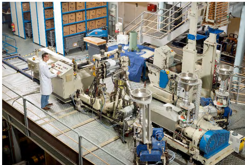
Production of multi-layer bioplastic sheets
