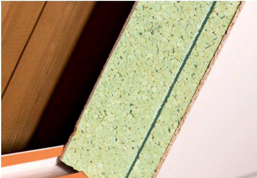
Biofoam isolation material (PLA-based polystyrene, Bewi-Synbra)
