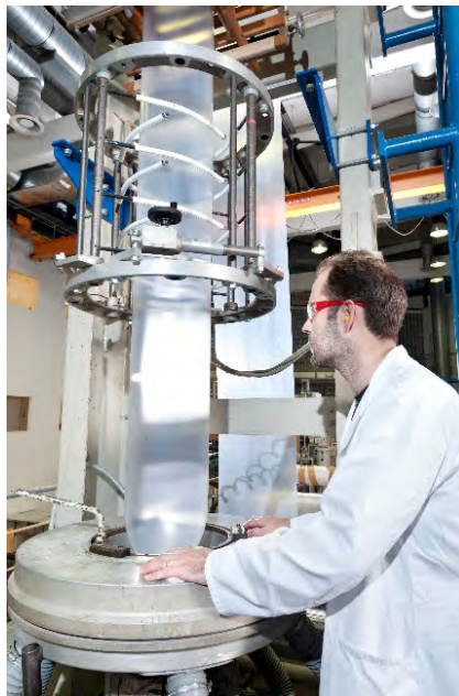
Production of starch-based film
