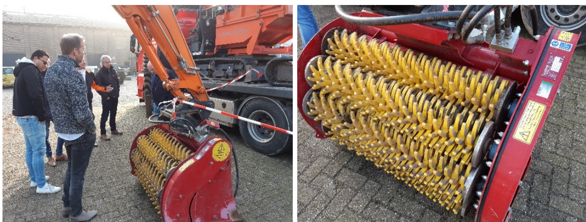
Figure 9 Mobile crane with bucket and rotating 'fingers' for digging and sifting. The soil falls through the bucket while larger segments (>2 cm) remain inside.
