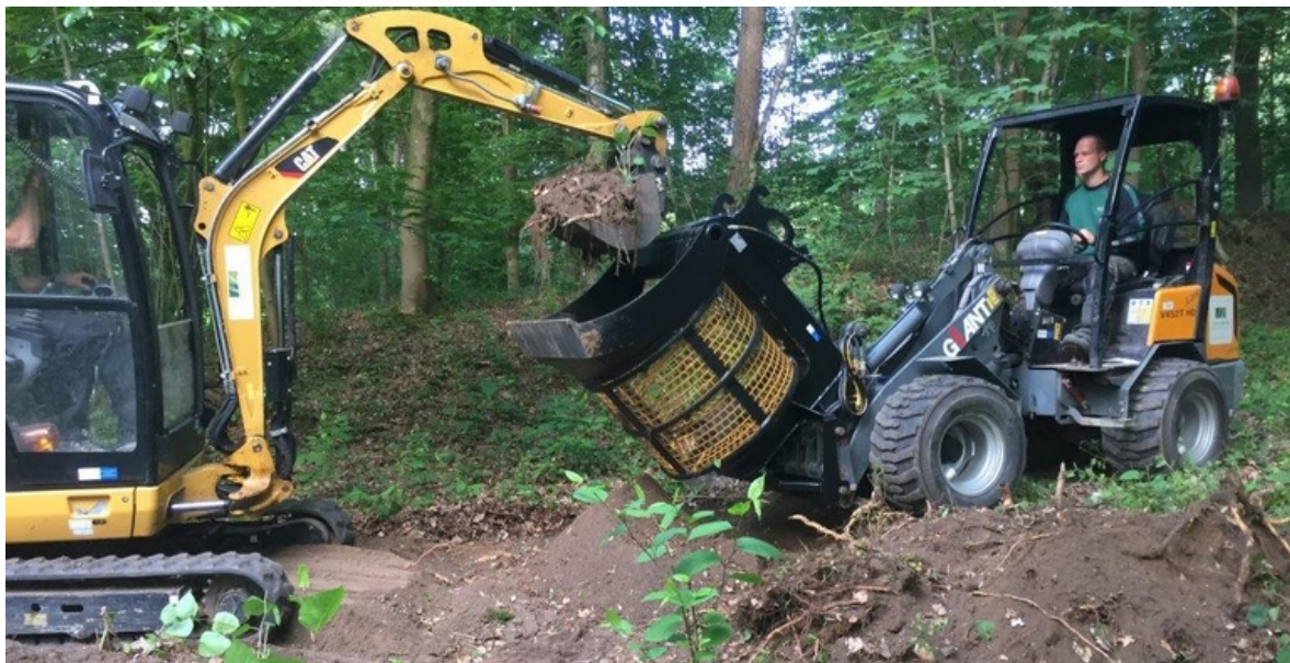
Figure 8 Machine digging and sifting (drum sieve) of Asian knotweed rootstocks.
