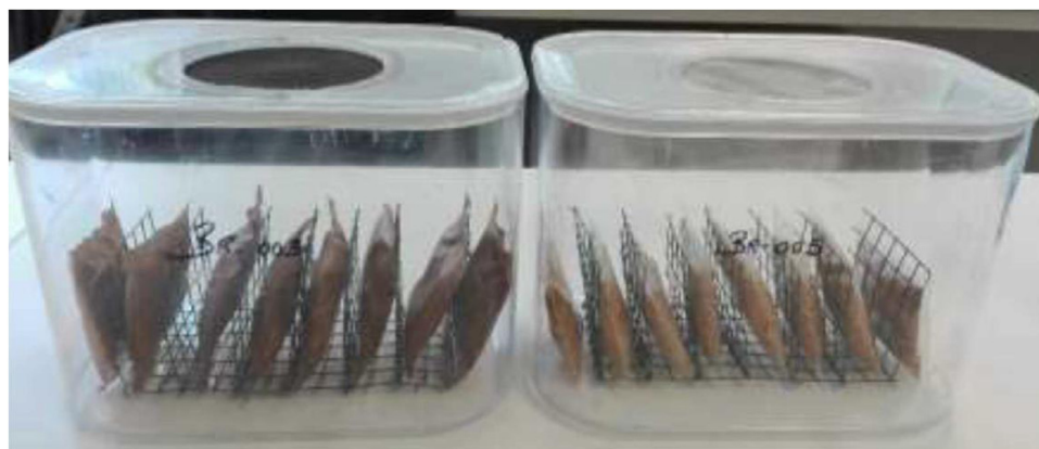
Fig. 6. Plastic box with the bags containing food for testing insect repellence (left box: HDPE-EAL; right box: HDPE-ref.).
