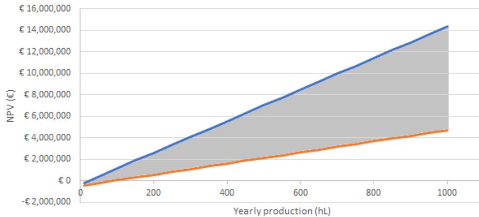
Appendix figure 1. Possible values of NPV for additional capacity, based on settings in Table 3 for a yearly production size between 50-1000 hL.
