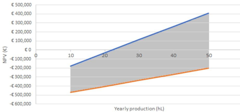
Appendix figure 2. Possible values of NPV for additional capacity, based on settings in Table 3 for a yearly production size between 10-50 hL.
