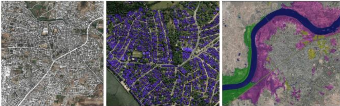
Figure 5: Three examples featuring subsequently the road extraction, building detection and land cover classification challenge datasets within the Deepglobe challenge. Source [25]
