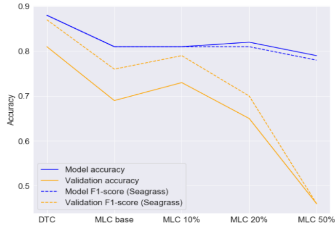
Figure 38. Comparison between model and validation accuracies of the DTC and MLC models in classifying Seagrass and non-Seagrass. The F1-scores of seagrasses are also plotted in this figure.
