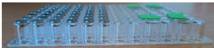
Figure 7.2. Magnet plate to pull down the streptavidin beads. Only half of the plate will contain beads so there is no need for a full plate of magnets.
