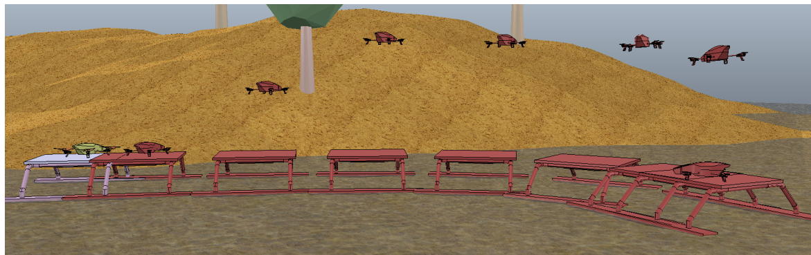
Figure 17. Ghost sequence of a VTOL manoeuvre in V-REP. Starting from the rightmost ghost, where the quadcopter is starting take off, to the leftmost, where the landing on the moving platform is achieved. The ghosts are one second apart from each other.
