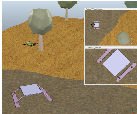
Figure 6. Screenshot of the V-REP environment in a lake scene. V-REP allows for environment mock-up models and multiple camera views for simulation and/or visualization.
