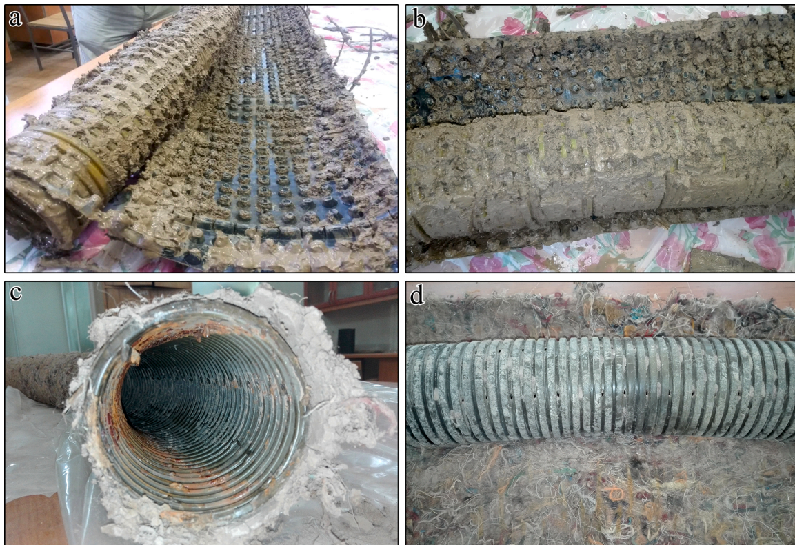
Fig. 5. Excavated drainpipes at the end of the experiment, Hydroluis (a, b) and PP450 (c, d).
