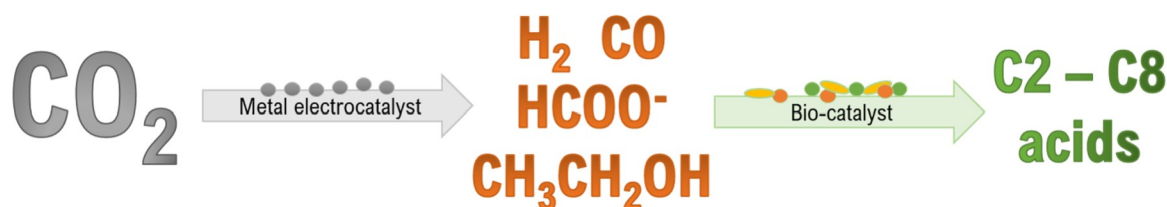
Scheme 1. Schematic of envisioned catalytic cooperation (in sequence) for the conversion of \text{CO}_2 . Intermediate products, including reduced \text{CO}_2 and electrocatalytically-produced hydrogen, are formed by a metal electrocatalyst, and can be further converted to longer carbon chains by a mixed culture of microorganisms (bio-catalyst).
